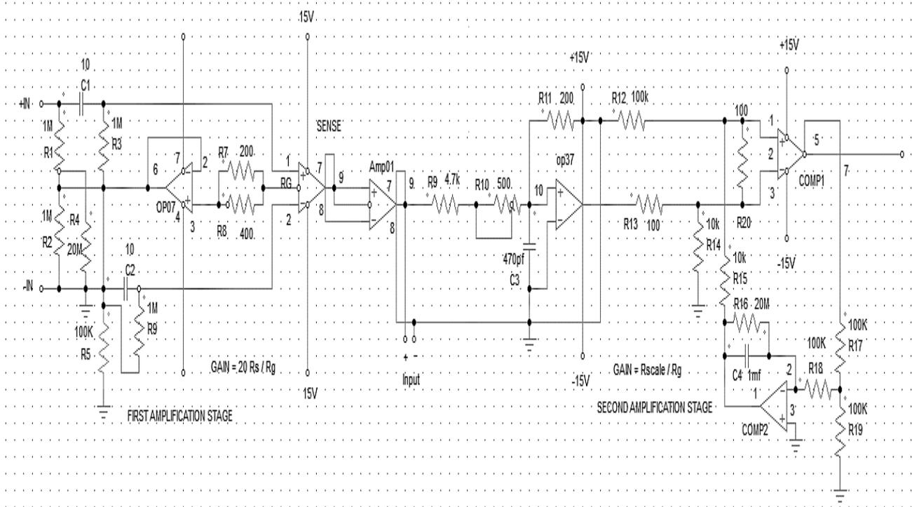
**Fig 3: Amplification Circuit for Brain Wave Processing Stage**
