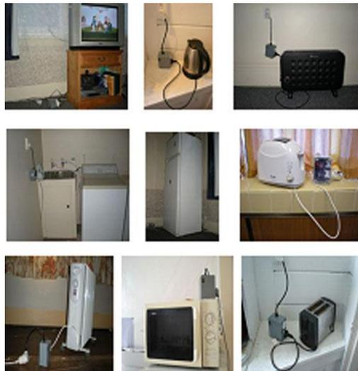
*Fig. 2 shows different appliances connected to the developed smart sensing system.*
