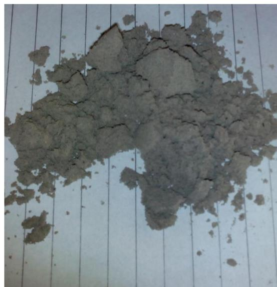
**Figure 2: Image of Thermal power plant fly ash**
