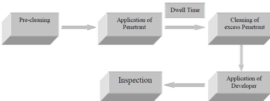
*Fig -8: Flow chart of dye penetrant process*
