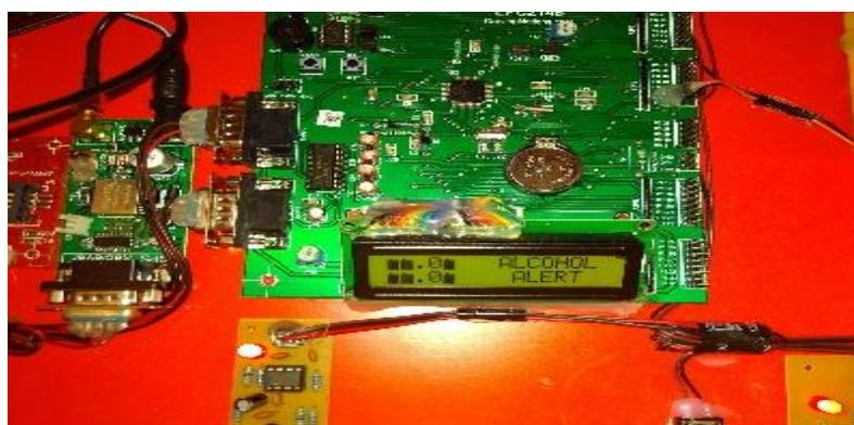
Fig 4: Alcohol alert on LCD
