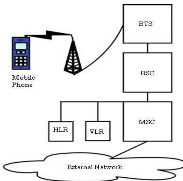
*Fig 1 - GSM Architecture*
