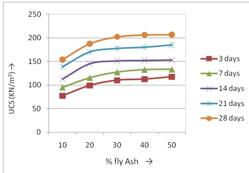
**Fig. 2 :** Variation of UCS with % of fly ash content and curing days
