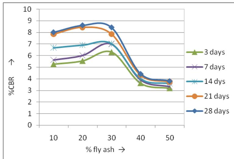
Fig. 4 : Variation of CBR value (unsoaked) with % of fly ash and curing days
