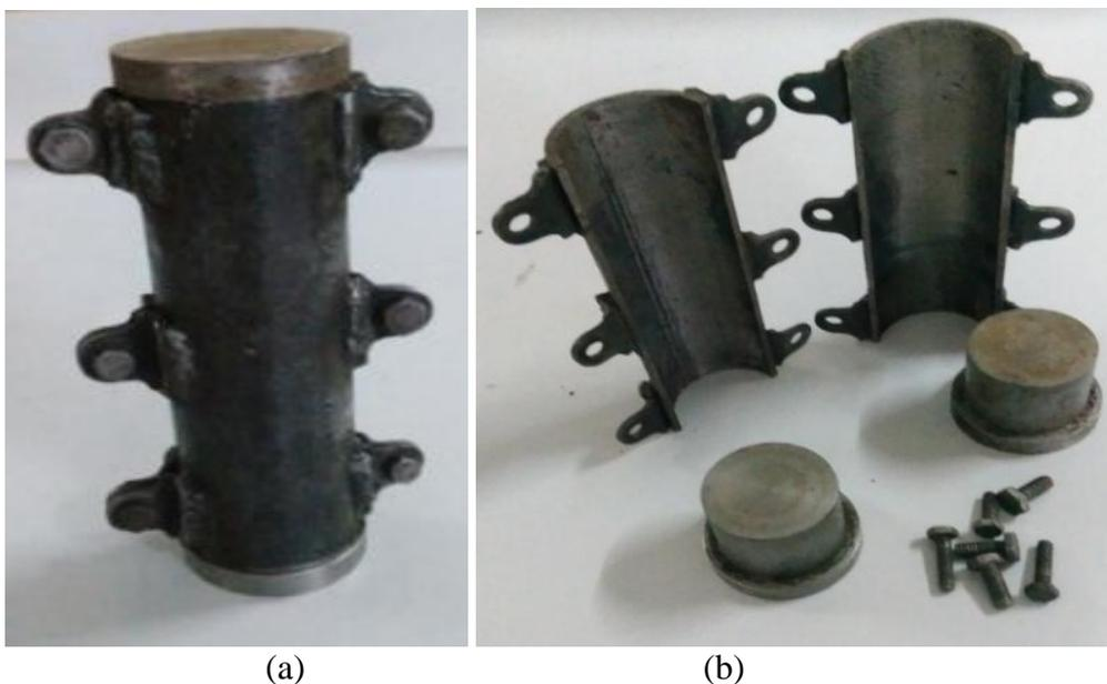
*Fig. 1 (a) &(b) : Static Compaction Mould for UCS test of Size 5.0 cm dia. x 10.0 cm height with plunger*
