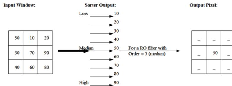
**Figure 2- Median Filtering**
