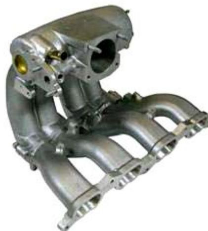
Figure1.Intake Manifold [1]
