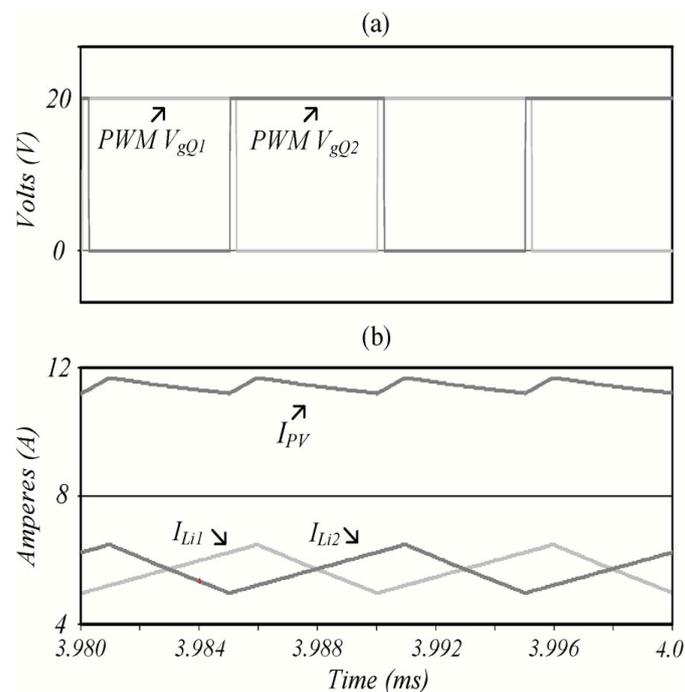
Figure 5. Simulation results of the input of the dc/dc converter. (a) Input switches' driving signals, (b) inductors' input currents  $I_{Li1}$  and  $I_{Li2}$ , and total input current ( $I_{PV}$ ).
