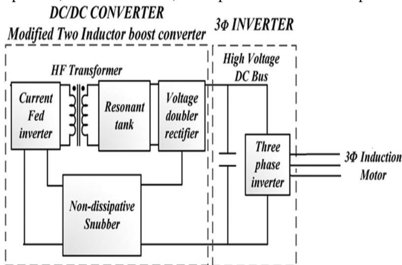
*Figure 1. Simplified block diagram of the proposed system*
