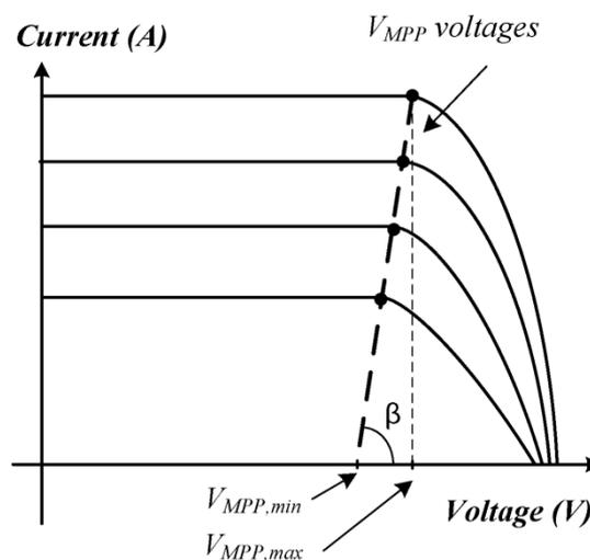
Figure 3 .  $I-V$  characteristic curves for a typical solar panel.
