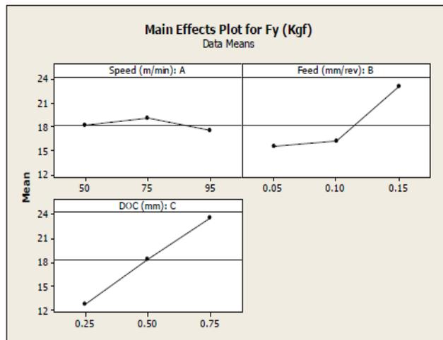
Figure. 2.4(A) Effect of Cutting Parameters on cutting force
