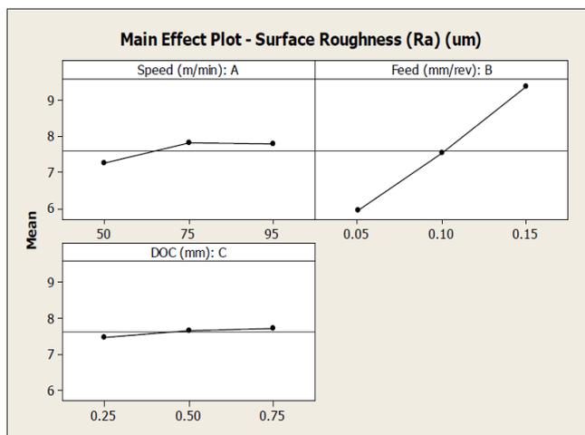
Figure. 2.4(B) Effect of Cutting Parameters on surface roughness
