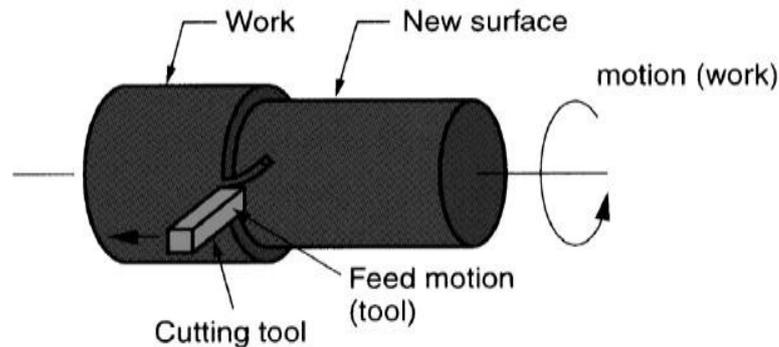
Fig. 1: Turning operation
