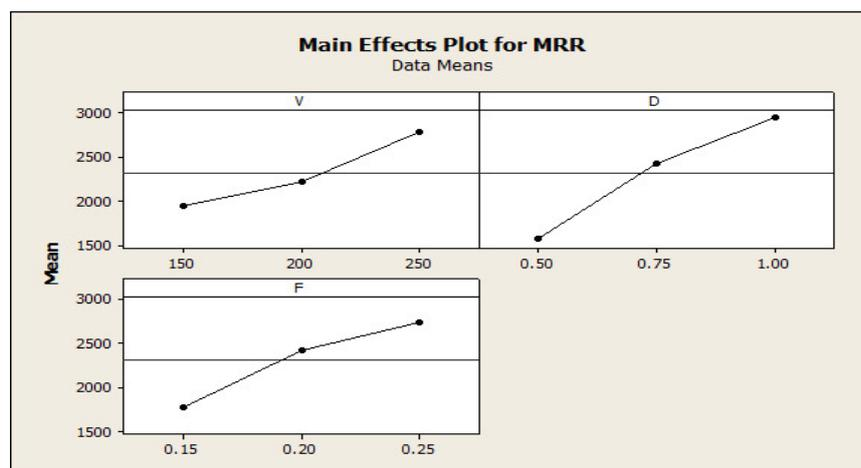
Figure: 2.2(c): Effect of Material Removal Rate
