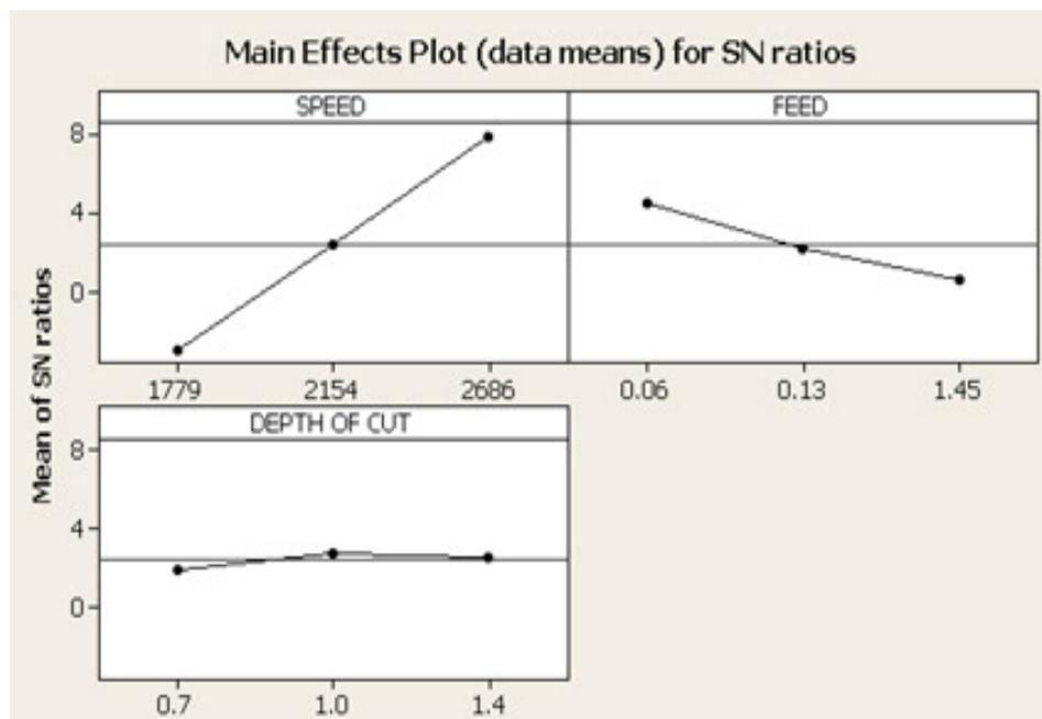
Figure: 2.1 effect of CBN Tools on speed, feed and depth of cut
