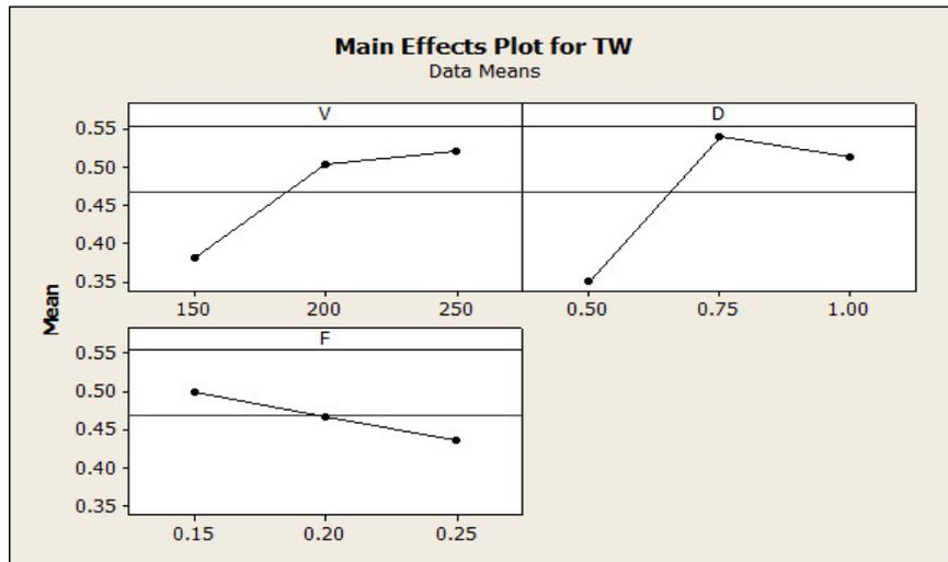
Figure: 2.2(a): Effect of Toolwear Rate
