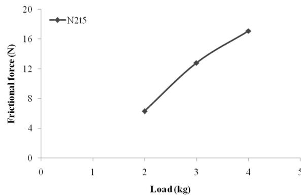
**Fig. 6 Frictional behavior of SAE 4340 Steel at N1 Speed**
