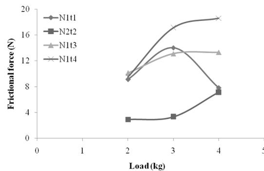
**Fig. 4 Frictional behavior of SAE 4340 Steel at N1 Speed**
