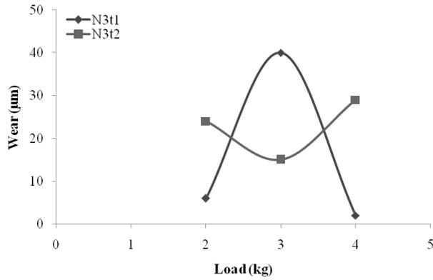
**Fig. 7 Wear of SAE 4340 Steel at N1 Speed**
