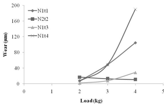
**Fig. 3 Wear of SAE 4340 Steel at N1 Speed**
