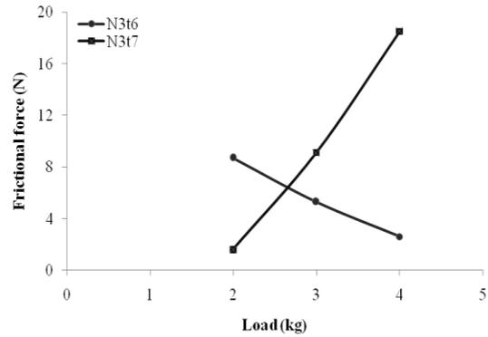
**Fig. 8 Frictional behavior of SAE 4340 Steel at N1 Speed**
