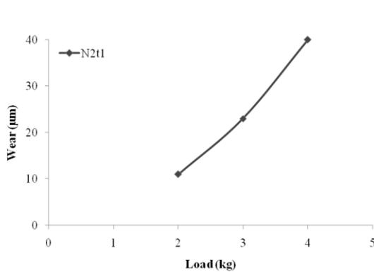
**Fig. 5 Wear of SAE 4340 Steel at N1 Speed**
