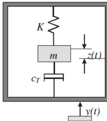
Fig. 1 Model of linear, inertial generator
