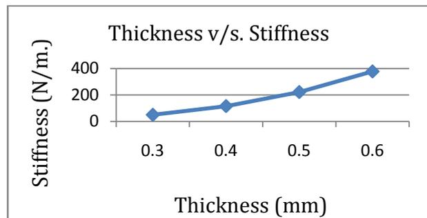
*Fig. 2 Graph of thickness V/s Stiffness*
