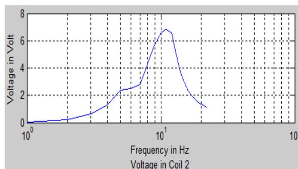
**Fig 6: Graph of frequency V/s Voltage in coil 2**
