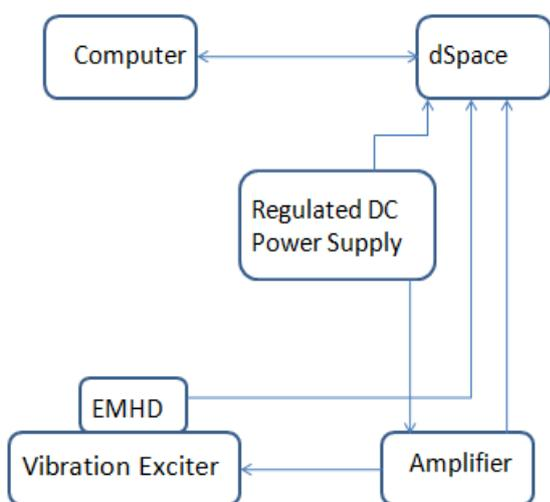
*Fig 3: Schematic diagram of set up*
