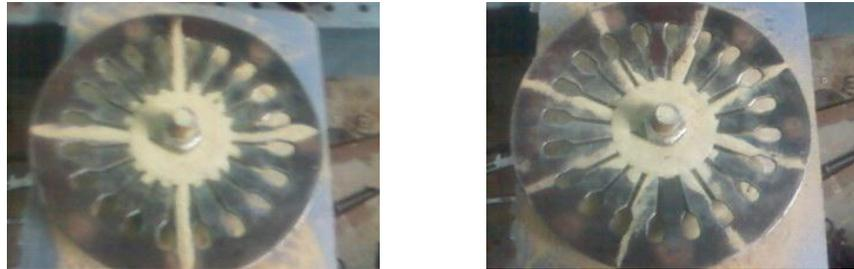
Fig.7 Mode Shape Showing Two Nodal Diameters & Four Nodal Diameters
