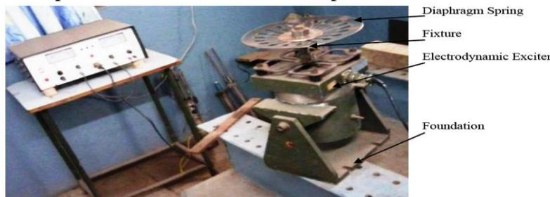
Fig. 6 Experimental Set Up For Exciter
