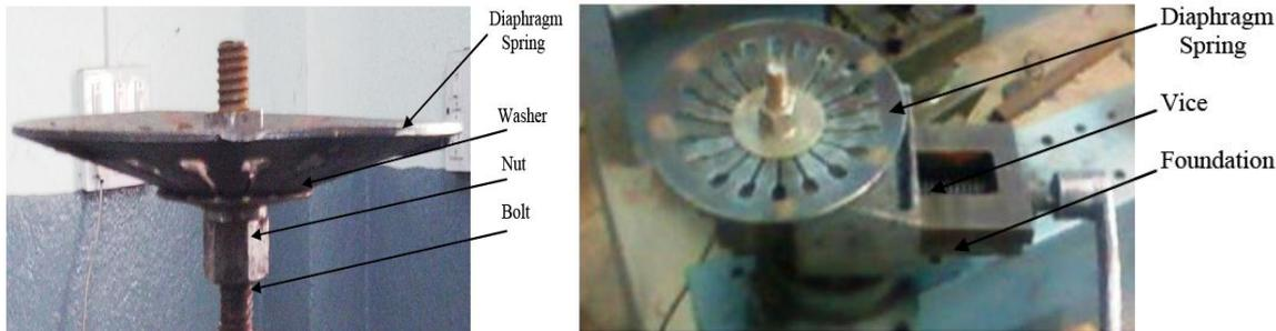
*Fig. 2 Clamping Details of Test (Front View) Fig. 3 Clamping Details of Test Specimen (Top View)*
