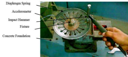
Fig. 4 Experimental Set Up for Impact Hammer FFT Test
