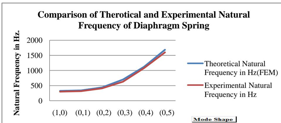
Fig. 8 Natural frequency plots for Theoretical results (FEM) and Experimental Results
