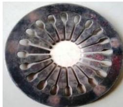
*Fig.1 Diaphragm Spring of Clutch specimen.*
