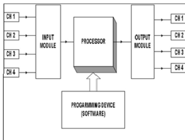
*Figure 1. Block Diagram of Typical PLC*
