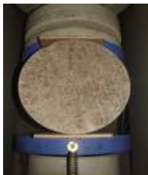
Fig.2 set up of splitting tensile strength
