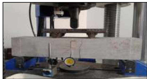
Fig.3 set up of flexural strength
