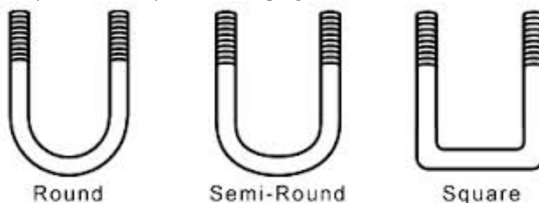
Fig 1. Formats of the bolts used in suspensions of vehicles (a)Round (b)Semi-round and c) Square.
