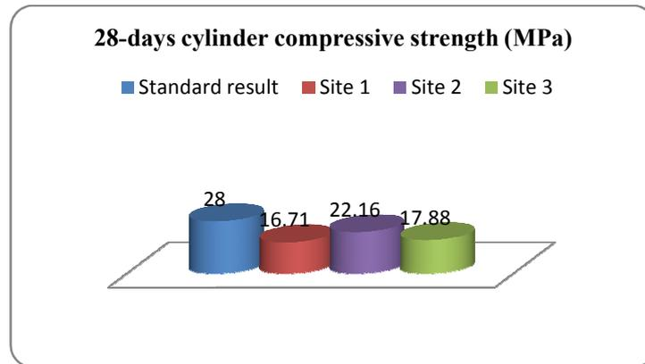
Figure 2. Comparison of cylinder compression test results
