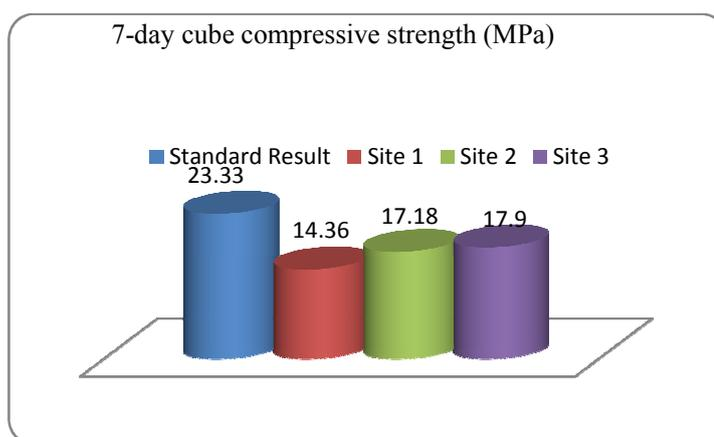
**Figure 1. Comparison of results of 7-days cube compression test**
