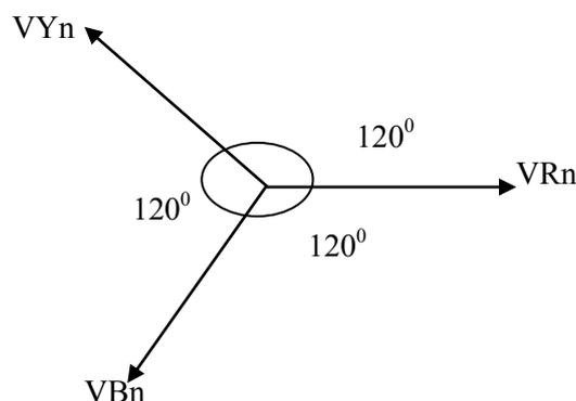
*Figure 1. Balanced 3-phase vector system*
