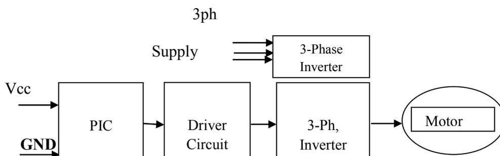
Figure 2. Architecture of proposed system
