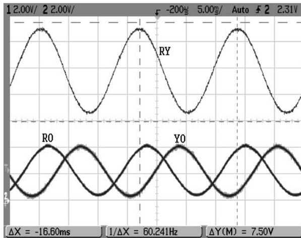
A) Sine PWM Generated Waveforms
