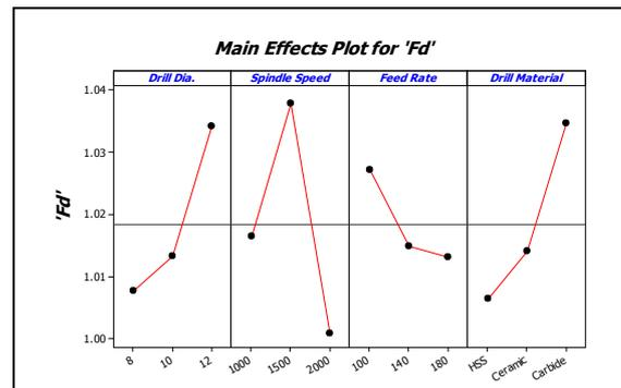
Figure 3. Main effects plots for Delamination factor ( $F_d$ )
