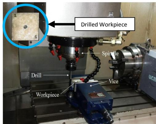
**Figure 2. Closed view setup of operation**
