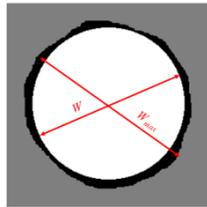
Figure 1. Measurement of maximum width of damage of a drilled hole in GFRP
