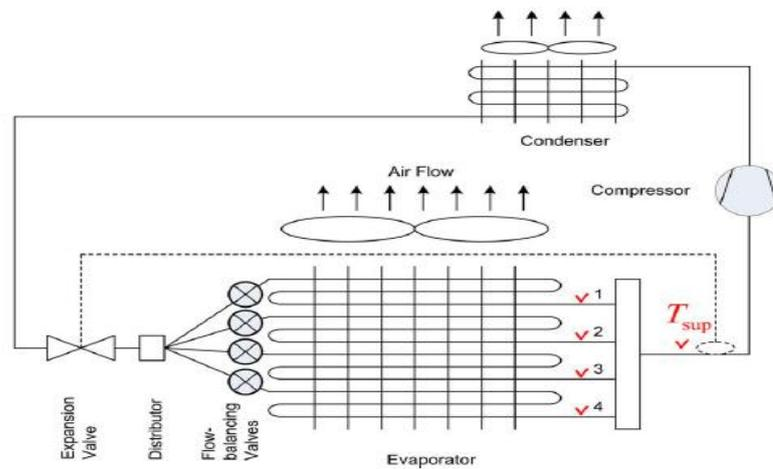
Fig. 1: Compression System with Hybrid Individual [6]
