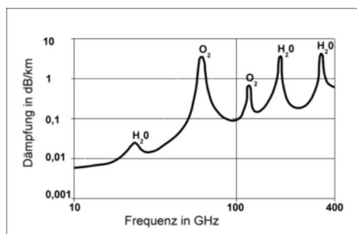
Figure 3: Atmospheric attenuation in dB/km as a function of frequency over the EHF band. Peaks in absorption at specific frequencies are a problem, due to atmosphere constituents such as water vapor (H<sub>2</sub>O) and carbon dioxide (CO<sub>2</sub>).
