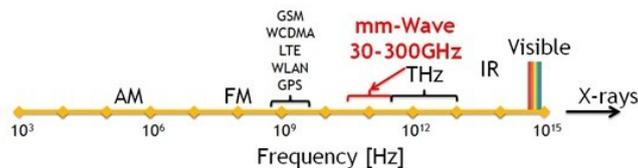
Figure 2. Millimeter wave frequency spectrum
