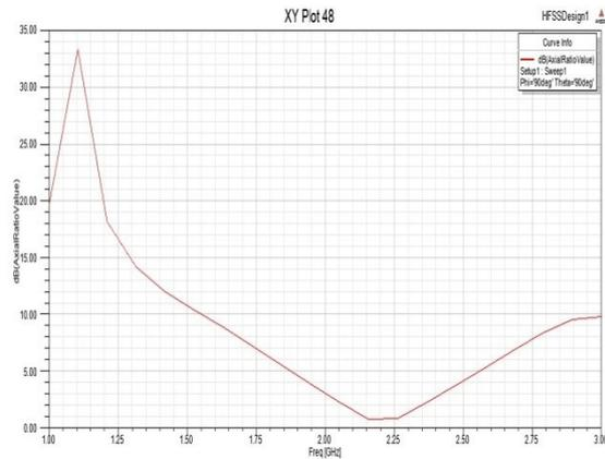
Fig. 4 Simulated Axial Ratio Bandwidth
