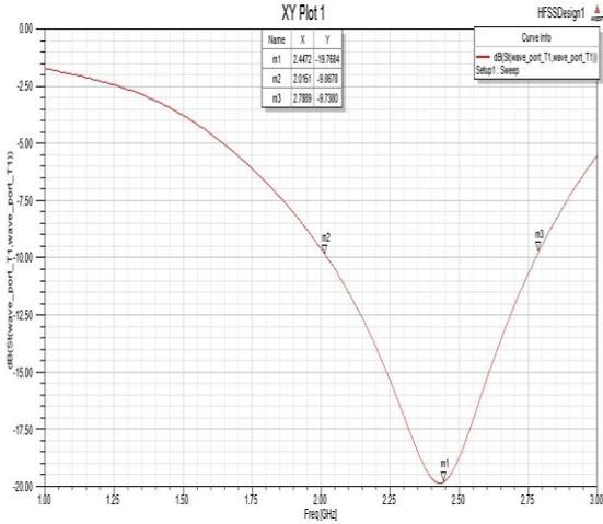
Fig. 2 Simulated S11 of the textile antenna
