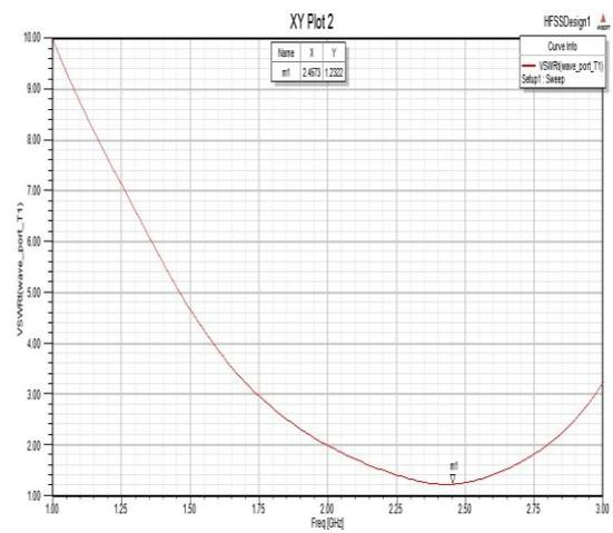
Fig. 3. Simulated VSWR of the textile antenna
