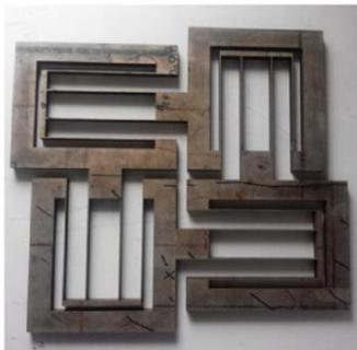
Fig 5: Manufactured XY Flexural Mechanism 1
