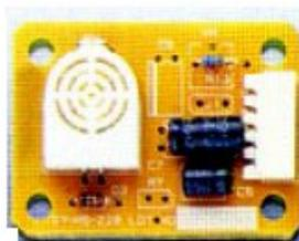
Figure 2. Humidity Sensor SY-HS-220
