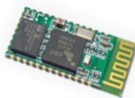
HC-05 module is an easy to use Bluetooth SPP (Serial Port Protocol) module, designed for transparent wireless serial connection setup.
