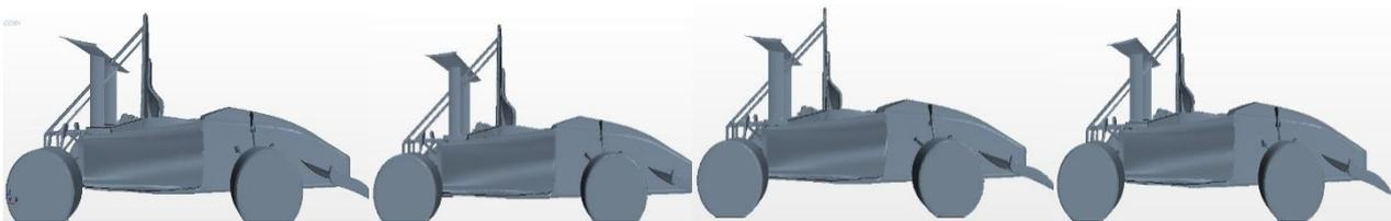
Fig. 4 Car with spoiler for  $-10^{\circ}$  and  $10^{\circ}$  angle of attack Fig. 5 Car with spoiler for  $-5^{\circ}$  and  $5^{\circ}$  angle of attack
