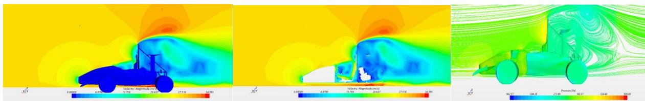
**Figure 8 Velocity Contours on the on the surface of the car and section view of computation domain**
