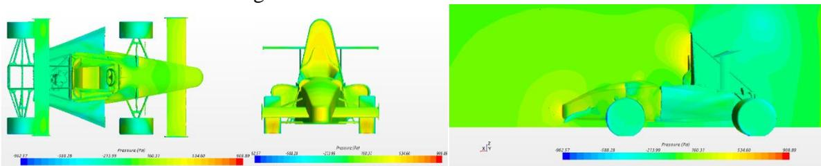
**Figure 7 pressure Contours on the surface of the car**
