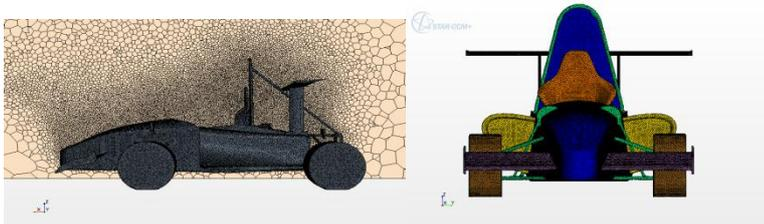
Fig. 6. Computational domain Fig. 7 Sectional view of mesh Fig. 8 Front view
