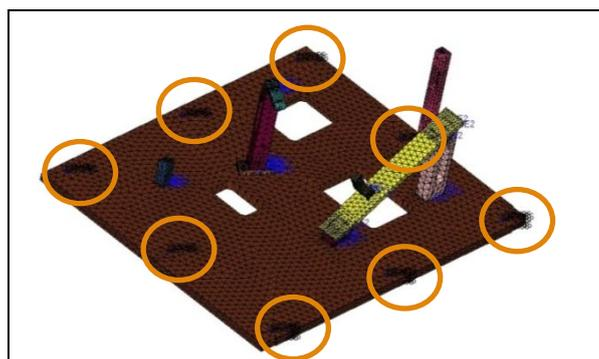
Fig. 1: Boundary conditions used in FEA
