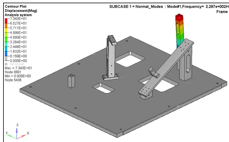
*Fig. 2: Mode shape for Final design of Headlamp fixture*
