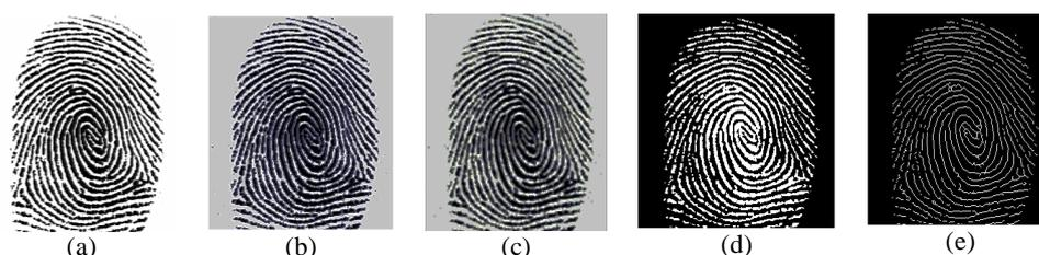
Figure 3: Results of Image Pre-Processing Techniques (a) Original Captured Image, (b) Histogram Equalization, (c) Noise Removal, (d) Binarization, (e) Thinning
