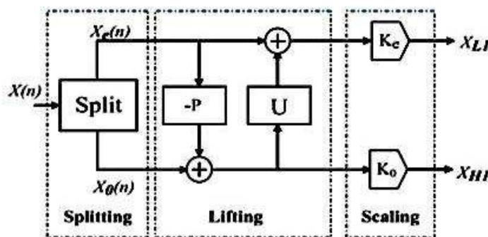
*Figure 1. The lifting-based Wavelet Transform.*
