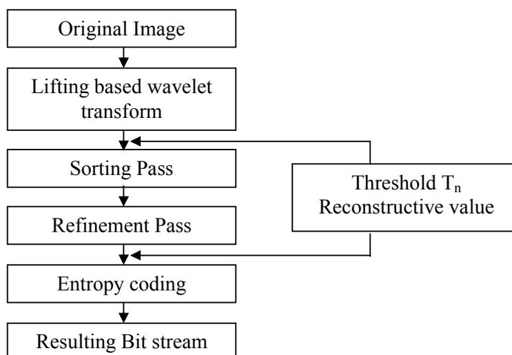
*Figure 2. Flow chart of SPIHT coding scheme*
