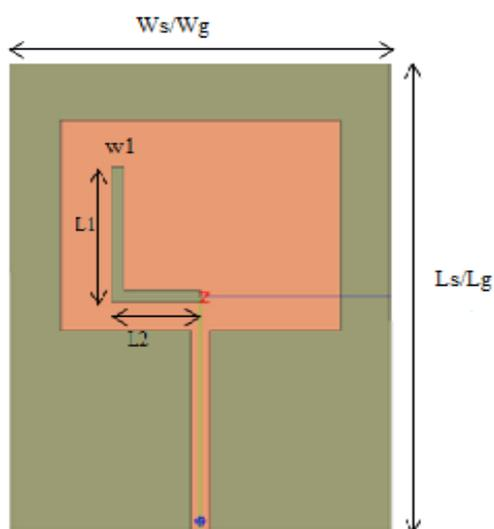
*Figure 1. The proposed dual band Microstrip antenna*
