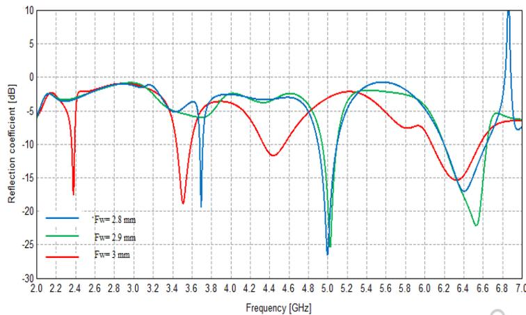
Figure 4. Effect of Micro strip position on S11
