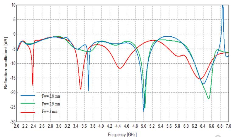
Figure 5. Effect of changing Feed width
