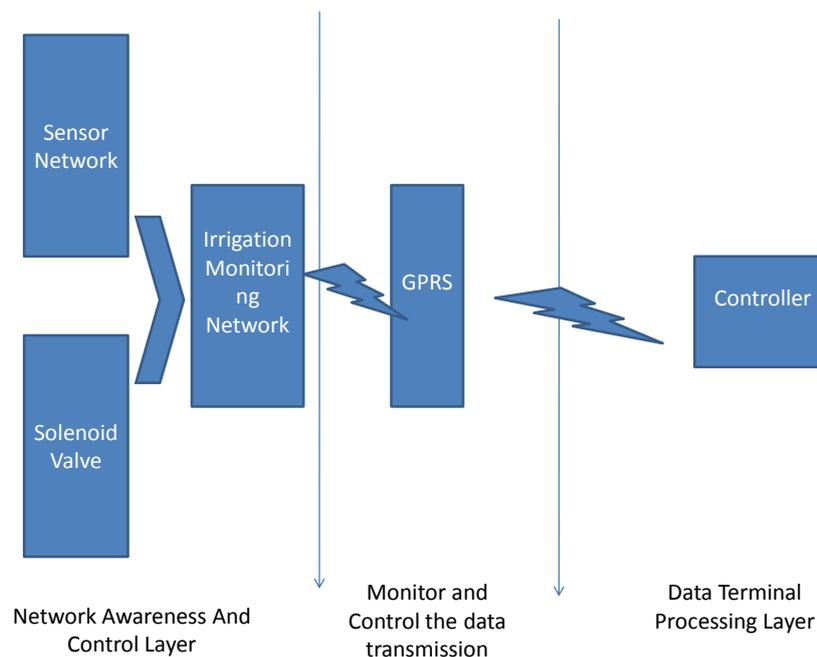
**Figure 2. Network constitution of irrigation system for precision agriculture**
