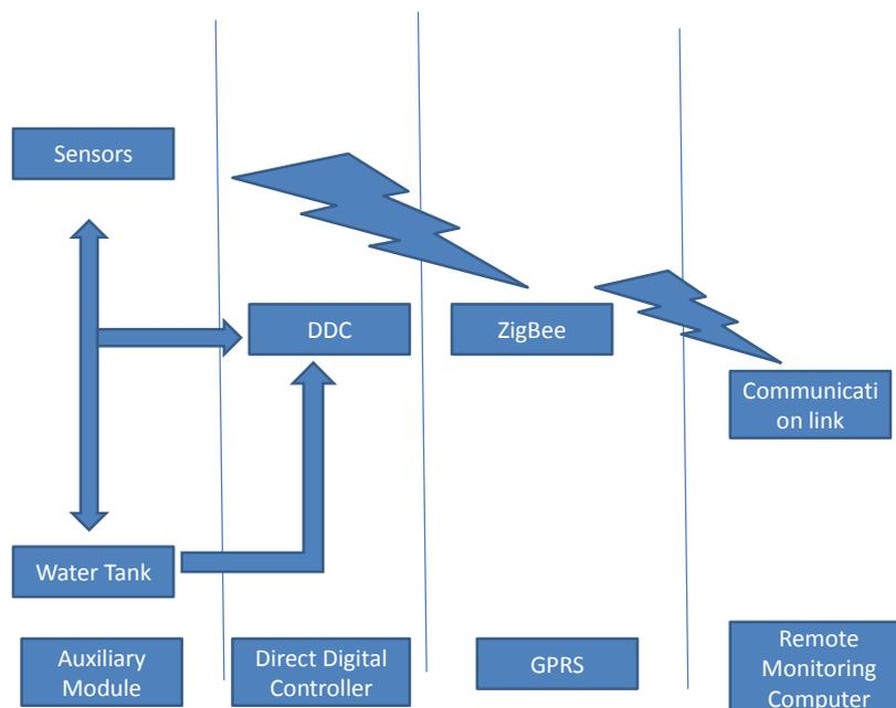
*Figure 1. Hardware system for precision agriculture Irrigation based on the Internet of things*
