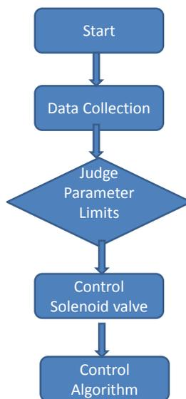
**Figure 3. Control flow chart of the system software running**
