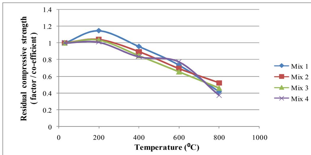
Figure 2. Variation of residual compressive strength V/s temperature
