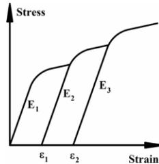
Fig. 2 Scheme of the method for measuring unloading Elastic modulus [2]
