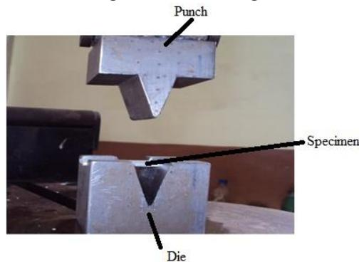
Fig. 4 Experimental set up for V bending
