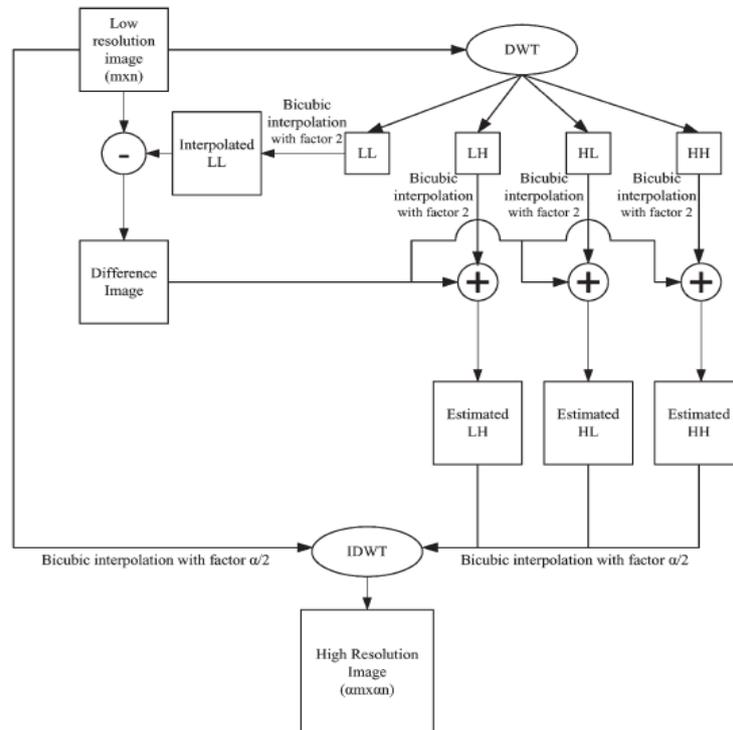
Figure 2 Block diagram of the proposed resolution enhancement algorithm.
