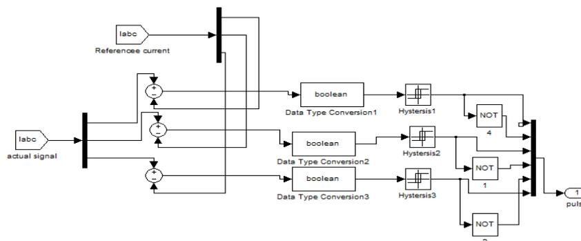
**Figure.5 Simulation diagram of hysteresis current control**
