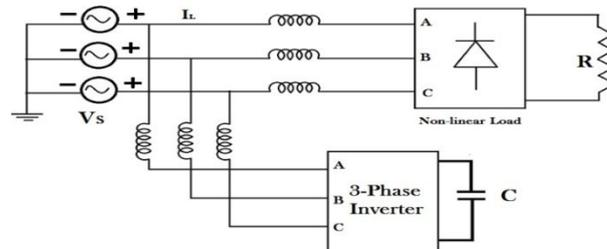
Figure.1 Three phase shunt active power filter
