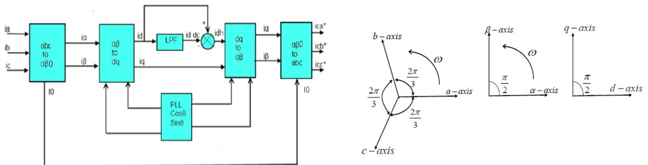
Figure.2 Block diagram of SRF based algorithm Figure.3 Reference Frame Transformation
