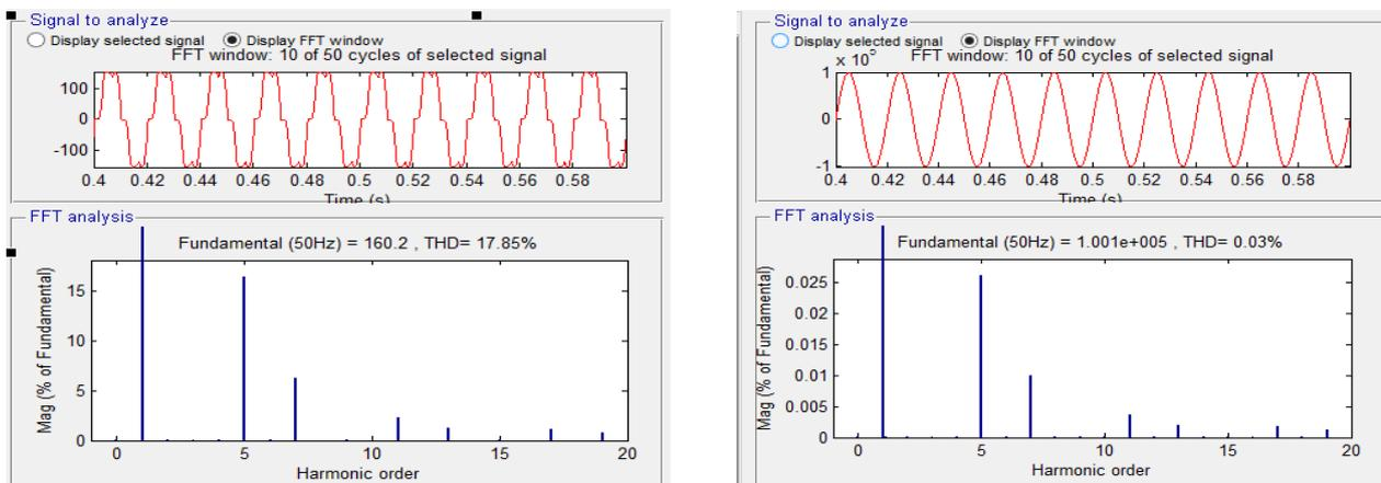
Figure.7 Source current and THD spectrum without SAF Figure.8 Source current and THD Spectrum with SAF
