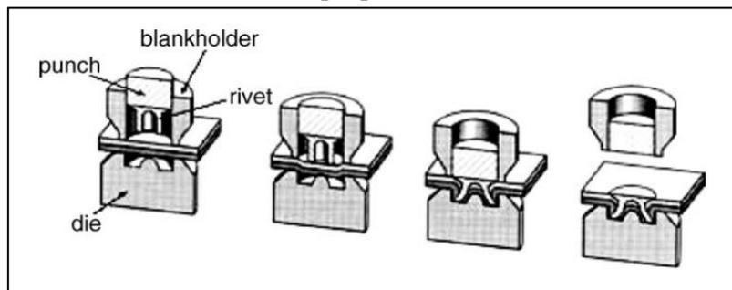
*Figure 1. Self-Pierce Riveting Process [2]*
