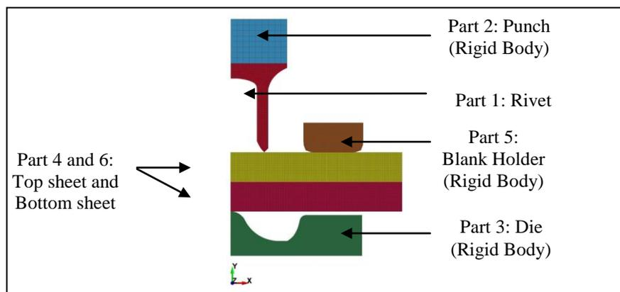
**Figure 3. Finite Element Model of Self-Pierce Riveting Process**
