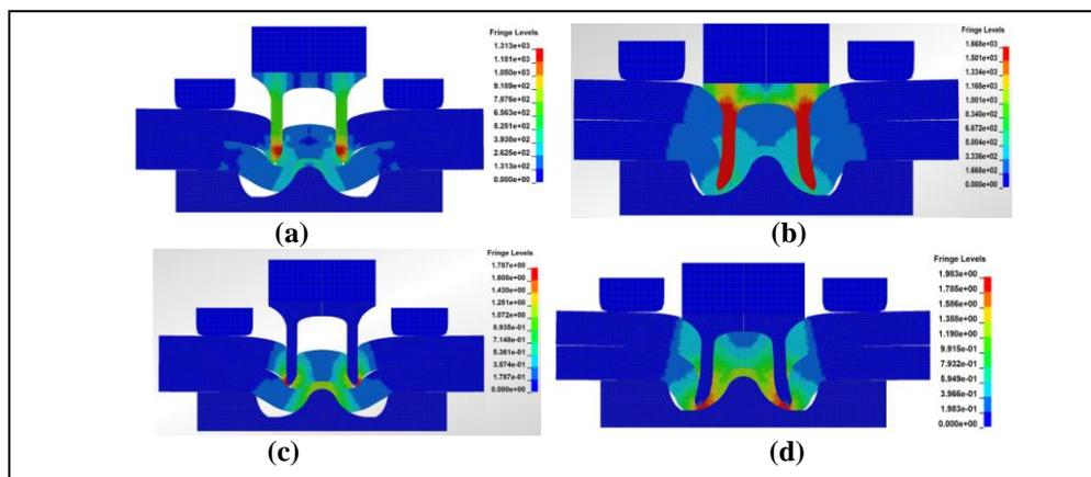
Figure 5. Effective Von-Mises stresses (a) 6.0 Sec (b) 10.0 Sec
