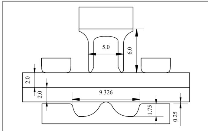
**Figure 2. Geometry and Dimensions of SPR Tools (All dimensions in 'mm')**
