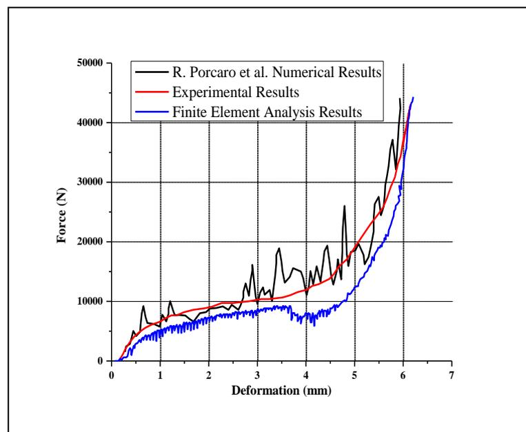
*Figure 4. Comparison of force vs. deformation graph*
