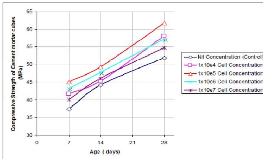
**Figure 1: Effect of bacterial cell concentration on the strength of concrete**
