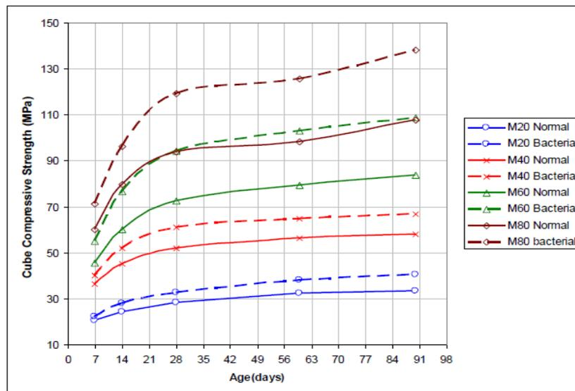
Figure 2: Strength development of a Normal concrete and Bacterial concrete
