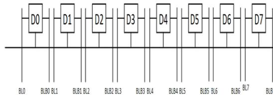
Fig.2 An 8 bit register using SRAM cell
