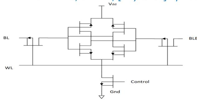
Fig. 3. Gated-Vdd to Reduce Leakage Power
