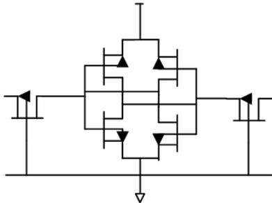
Fig. 1 Conventional 6T SRAM Cell
