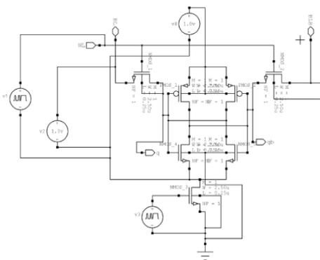
Fig. 4. SRAM cell with Gated Vdd
