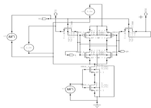
Fig. 5 SRAM cell with NMOS stack
