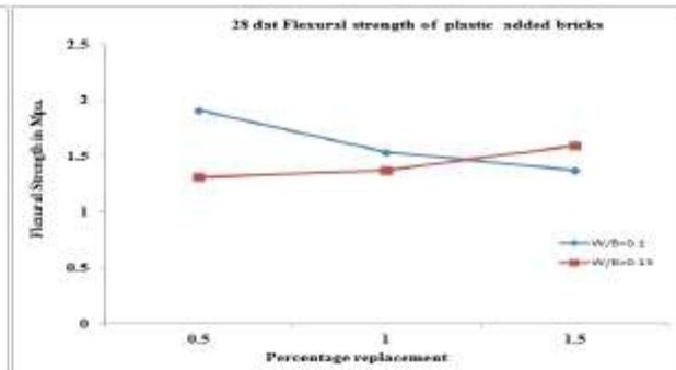
Figure 6. Flexural strength of GA added bricks
