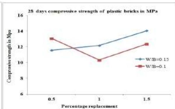
**Figure 4. Compressive strength of bricks with GA**
