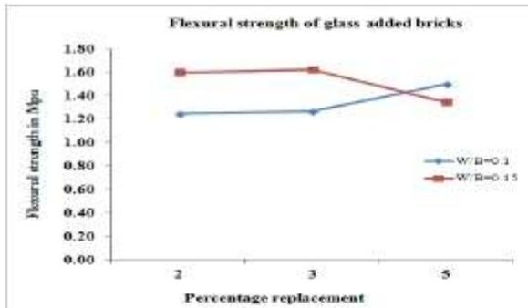
Figure 5. Flexural strength of WPA added bricks
