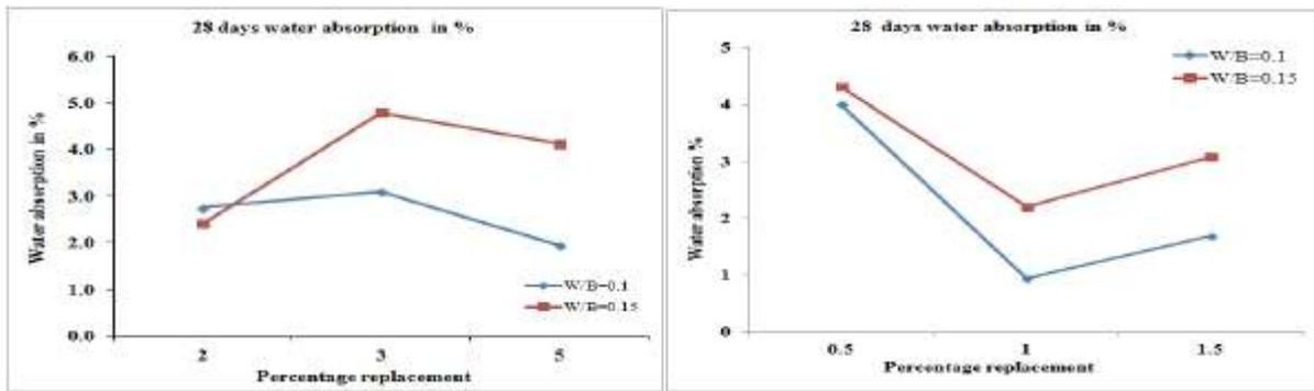
Figure 7. 28 day water absorption of WPA added bricks in % Figure 8. 28 day water absorption of GA added bricks
