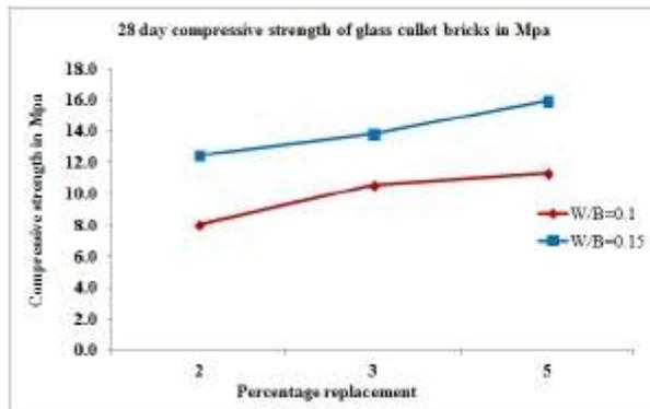
**Figure 3. Compressive strength of bricks with WPA**
