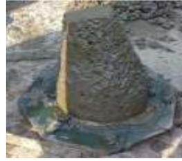
Figure 2: Slump of concrete at 5% GA.
