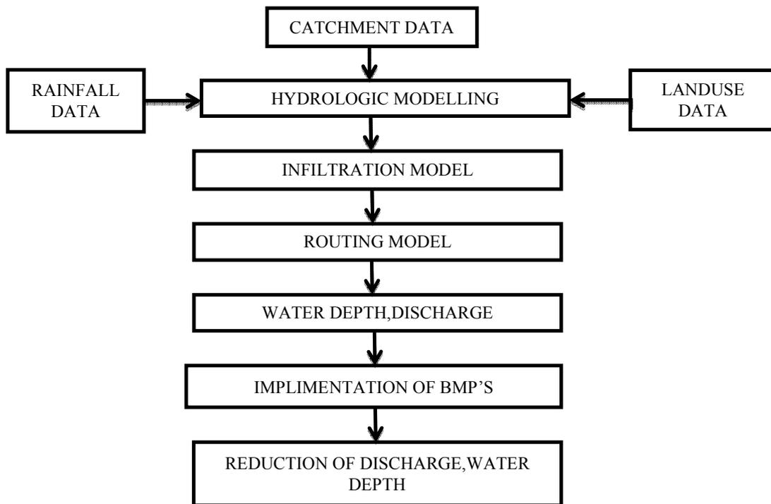
Figure 2. Conceptual framework by using SWMM
