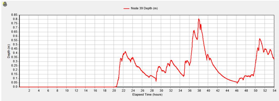
Figure 4. Depth simulation by using SWMM.
