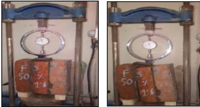
Figure6. Before and after failure pattern of brick triplet
