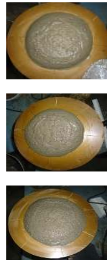
Figure2. Flow of Natural sand, Quarry dust and Foundry sand Mortar respectively
