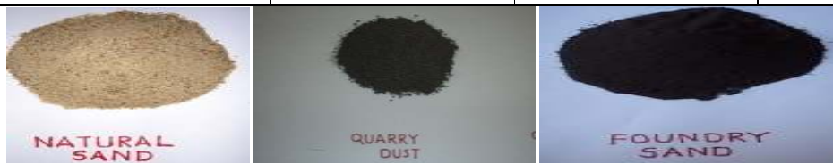
Figure1. Texture of Natural sand, Quarry dust and Foundry sand respectively
