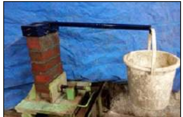
Figure7. Modified bond-wrench test setup
