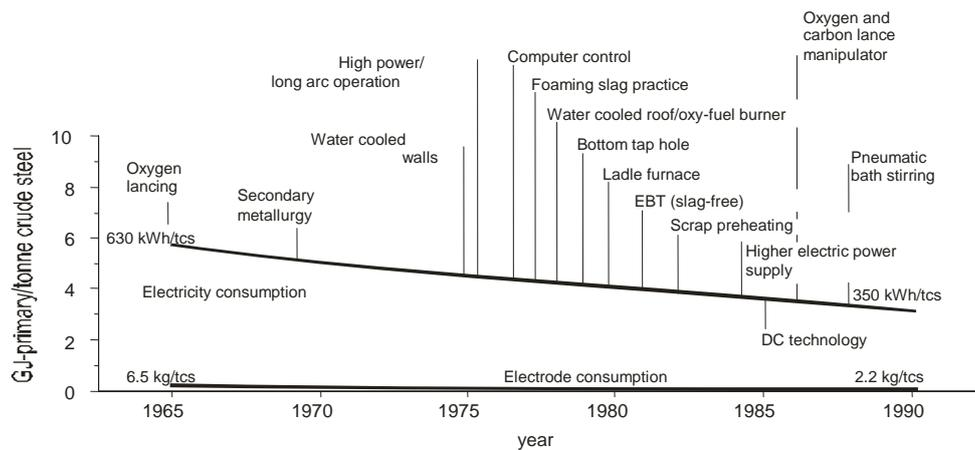
Fig. 1: Energy used by EAFs per tonne of crude steel
