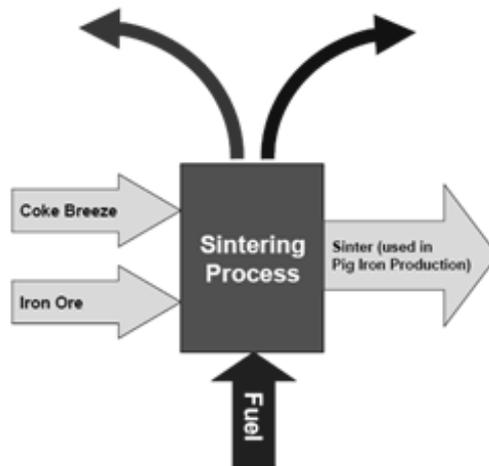
Fig. 2: Production Scheme of Sinter Production Process. Red Arrow Represents Combustion Emissions, Blue Arrow Represents Process Emissions
