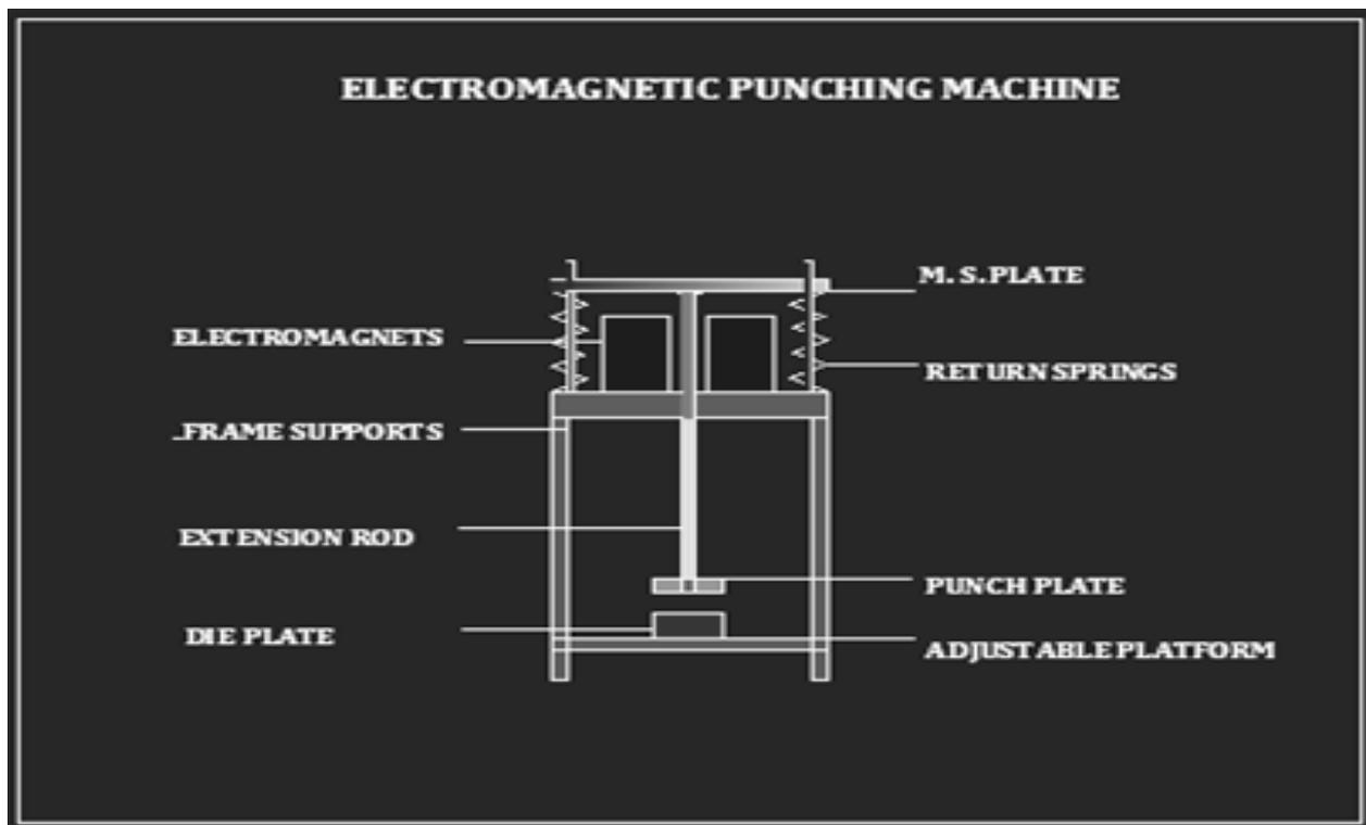
**Fig. 2 Electromagnetic Punching Machine**
