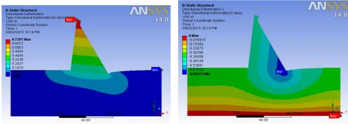
Figure 5. X & Y deformation in static analysis of dam with soil structural interaction
