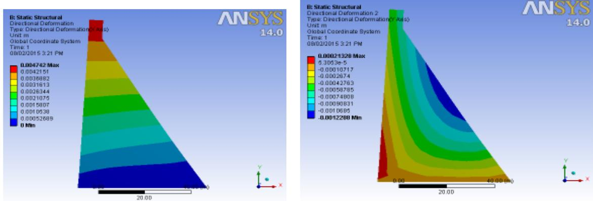
Figure 3. X & Y- deformation in static analysis of dam without soil structural interaction
