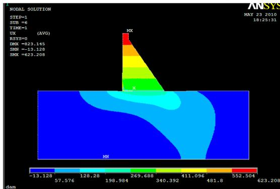
Figure 6. X - Displacement of gravity dam
