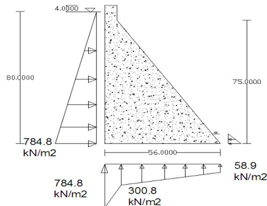
Figure 1. Various forces acting on gravity dam
