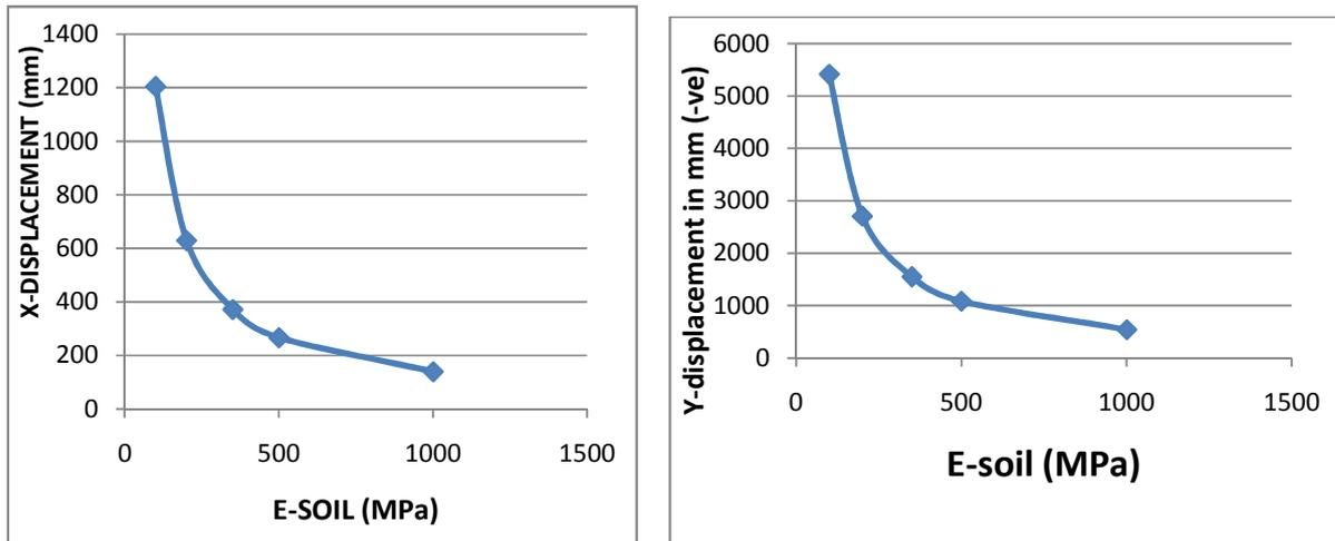
*Figure 10. The graph of X-displacement & Y-direction displacement*
