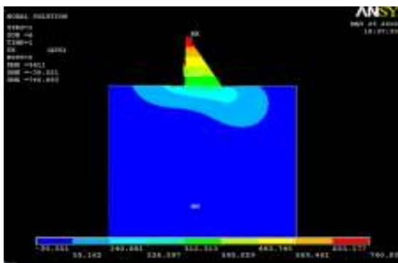
Figure 8. X - Displacement of gravity dam
