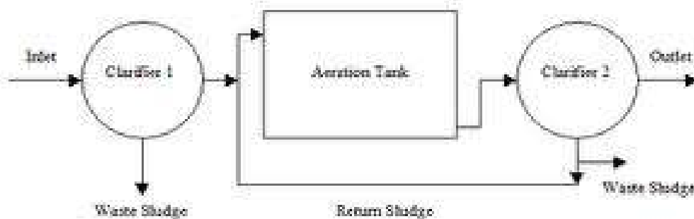
Fig.1 Schematic diagram of lab scale model of extended aeration system
