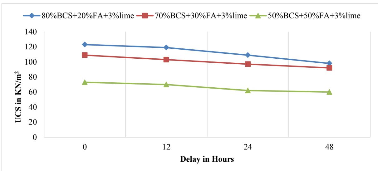
Figure 5. Variation of UCS due to delay in compaction of fly ash treated soil with 3% lime
