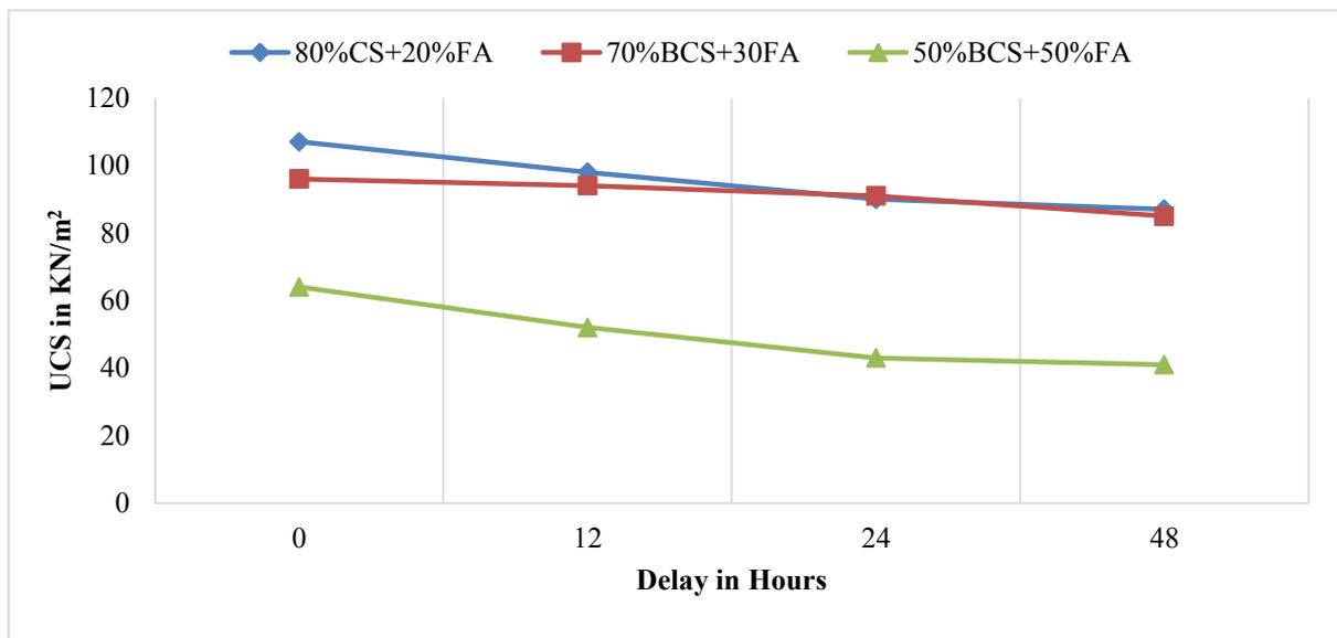
Figure 4. Variation of UCS due to delay in compaction of fly ash treated soil without lime
