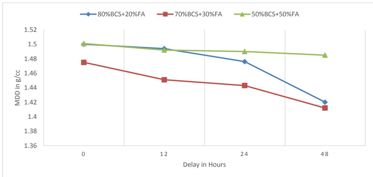
Figure 3. Variation of MDD due to delay in compaction of fly ash treated soil with 5% lime
