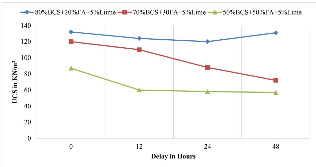
Figure 6. Variation of UCS due to delay in compaction of fly ash treated soil with 5% lime
