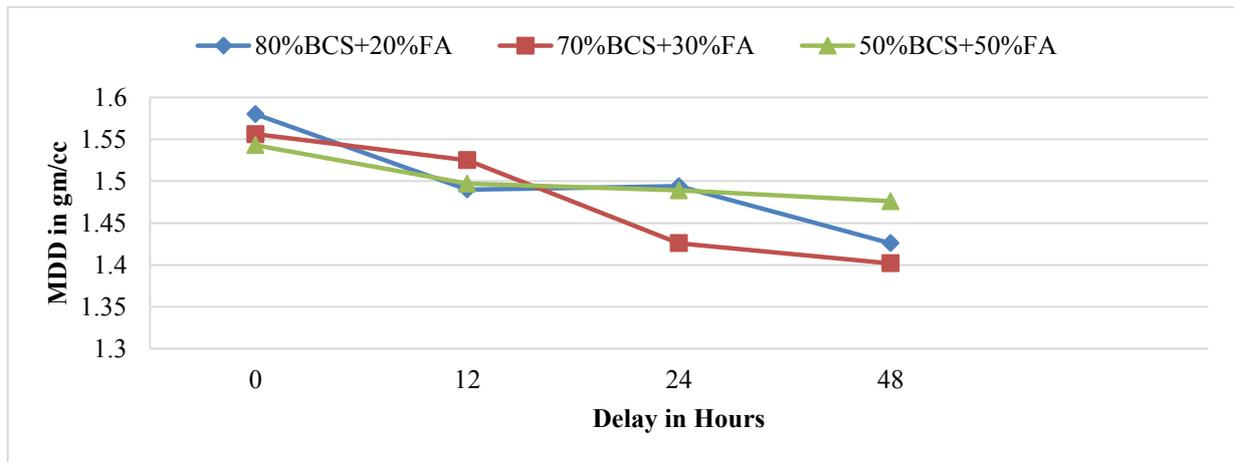
Figure 1. Variation of MDD due to delay in compaction of fly ash treated soil without lime
