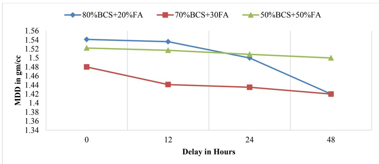
Figure 2. Variation of MDD due to delay in compaction of fly ash treated soil with 3% lime
