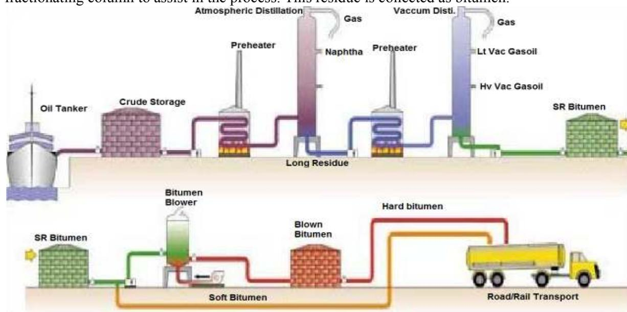
**Fig1.1 Manufacturing of Bitumen**
