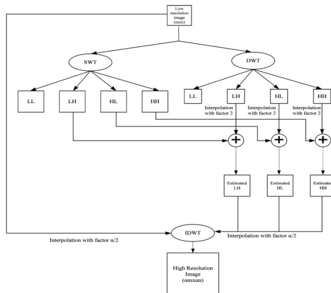
Figure 3. Block diagram of the proposed super resolution algorithm.
