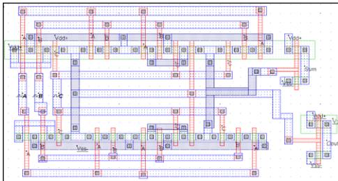
Figure 3. optimize layout of 28T full adder
