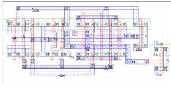
Figure 4. optimize layout of 24T full adder
