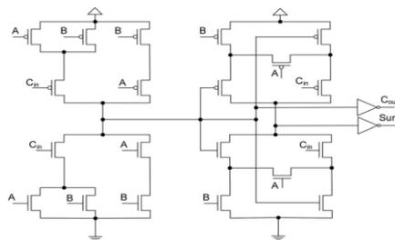
**Figure 2. 24T FA Mirror Based Full Adder**
