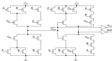
**Figure 1. Typical 28-transistor mirror FA**
